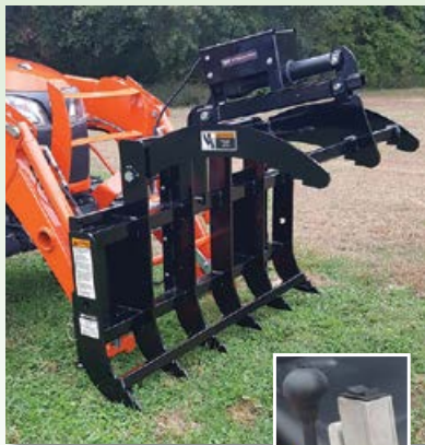
Grapple is controlled by a rocker switch mounted to the loader joy stick
