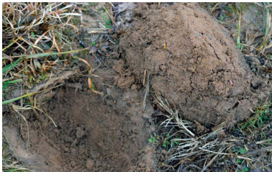
A wedge the size of the shovel is all that is needed to open the ground enough to take a good sample.
