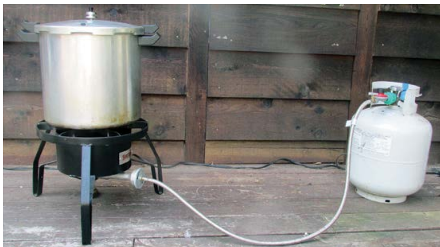
An outdoor canning set-up including a propane burner and steam pressure canner.
